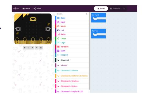
If you're using a Click Board<sup>™</sup> you'll see there is a section of dropdown toolboxes where you can find the exact Click board<sup>™</sup> you're using. In this case, we are using the Weather click which "senses" weather, so you can find it under the ClickBoards: Sensors toolbox category here:
