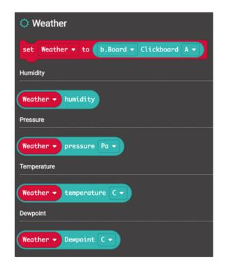
Since we only need to tell the b.Board one time where we plugged it in, we are going to drop this block into the "on start" block. The on start block runs all of the blocks you snap into it just one time, when you first power on your b.Board.
